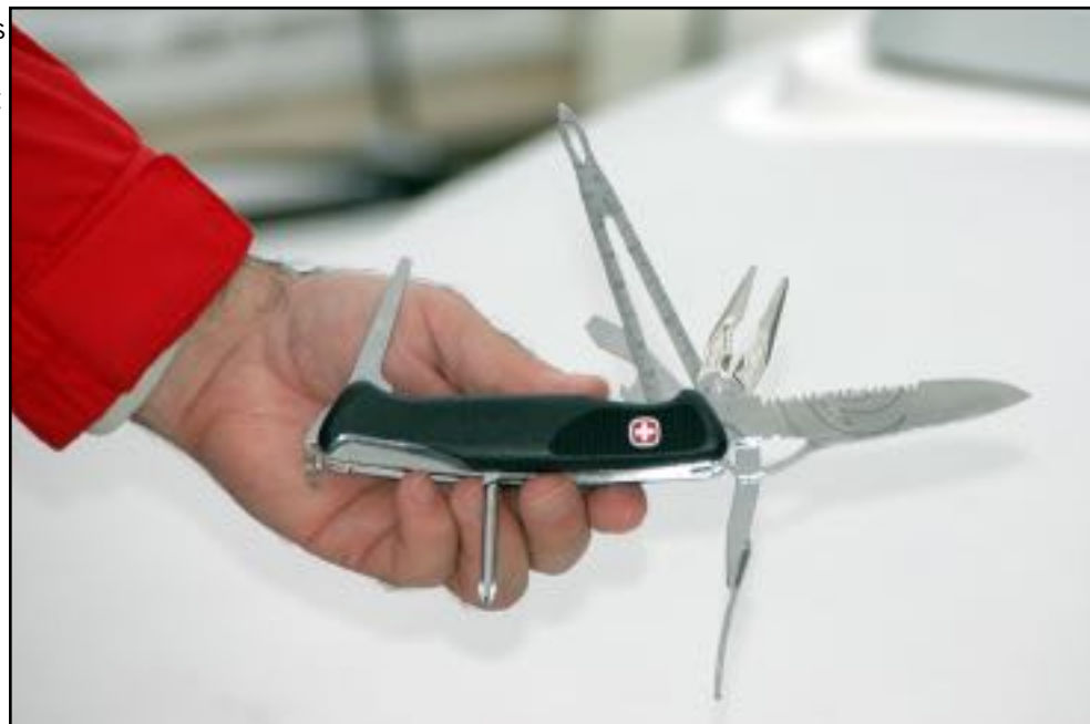
The Swiss-Army's Alinghi boasts a wire stripper, screwdrivers, reamer, awl, shackle opener, needle nose pliers, a reamer, a marlinspike, wire cutters and more. Photos by Marco Oquendo
