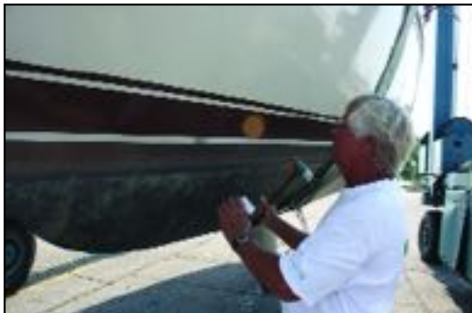
Surveyor Jack Morman of Morman Marine Surveyors tests the hull for water intrusion with a moisture meter and mallet.
